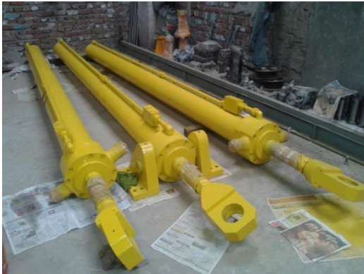
Radial Gate Servomotors for Karikyam Project
