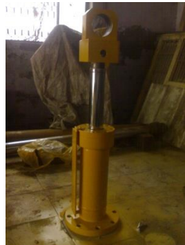
Guide Vane Servomotors for Vrindavan Project
